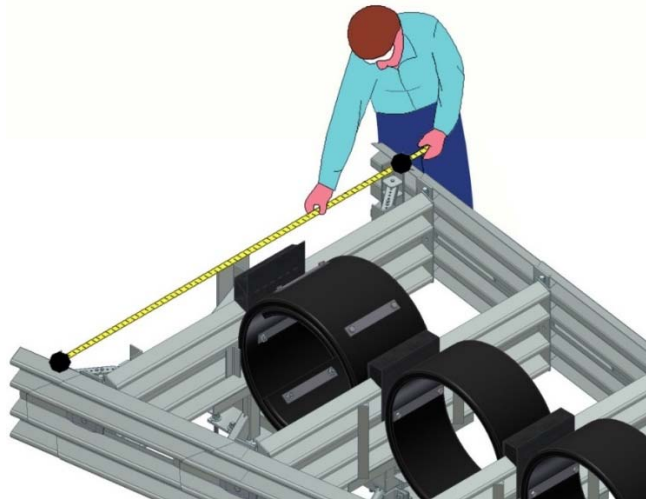
Figure 14 Width of System with Tension Strut Backup
